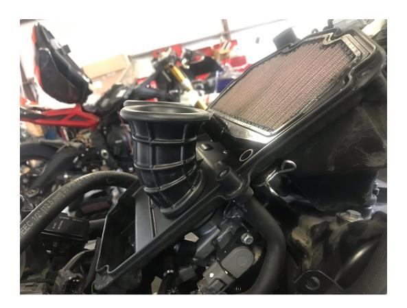
After removal of bottom air box half we investigated the throttle bodies. Although there is no FIM spec for throttle body bore the throttle bodies were modified compared to stock. The modified throttle bodies are 2.5 millimeters larger than the stock standard.
